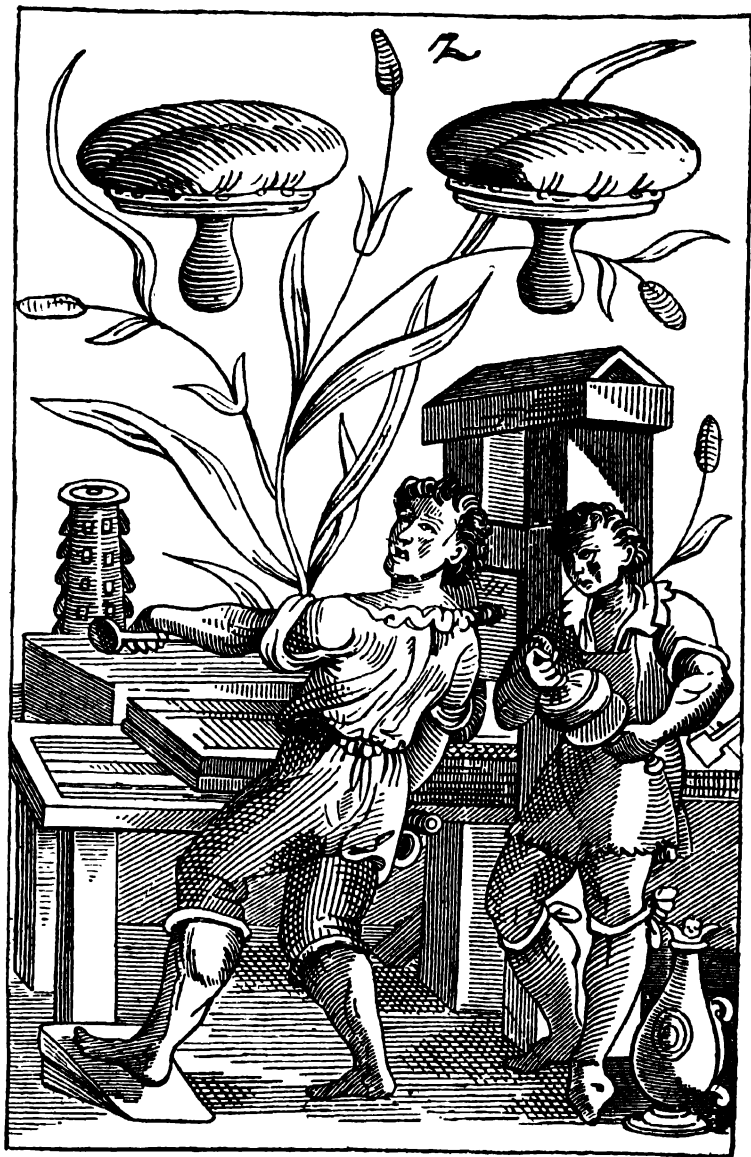
EARLY INK BALLS AND HAND PRESS FROM AN OLD PRINT BY JOSE AMMAN, 1568
